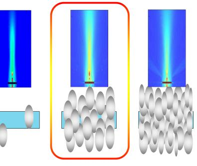
Tailor made coupling based on speciality polymer allows optimal ultrasonic intensity and residue free removal
