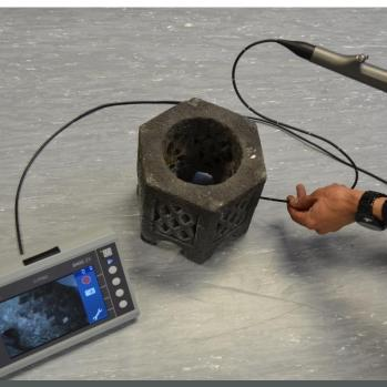
Recording of surface with scanner; voids with endoscope
