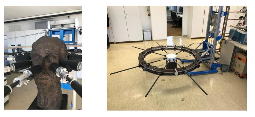
Scan ring with maximum 24 transducers and atomatic position acquisition Disadvantage - too rigid for most applications
